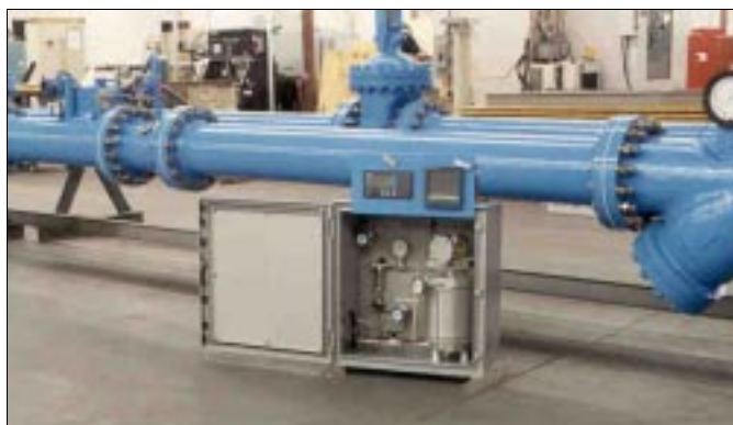
10" Natural gas fuel metering skid, referred to as "Big Blue" by our staff, just before shipment.
